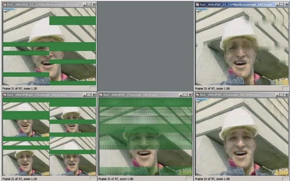
Figure 6 – Same aggregate bandwidth, number of packets and average packet size, and with 30% packet loss rate. *Top row*: standard coding. *Bottom row*: four multiple descriptions generated by separating odd/even lines and taking every other pixel; before and after concealment.
